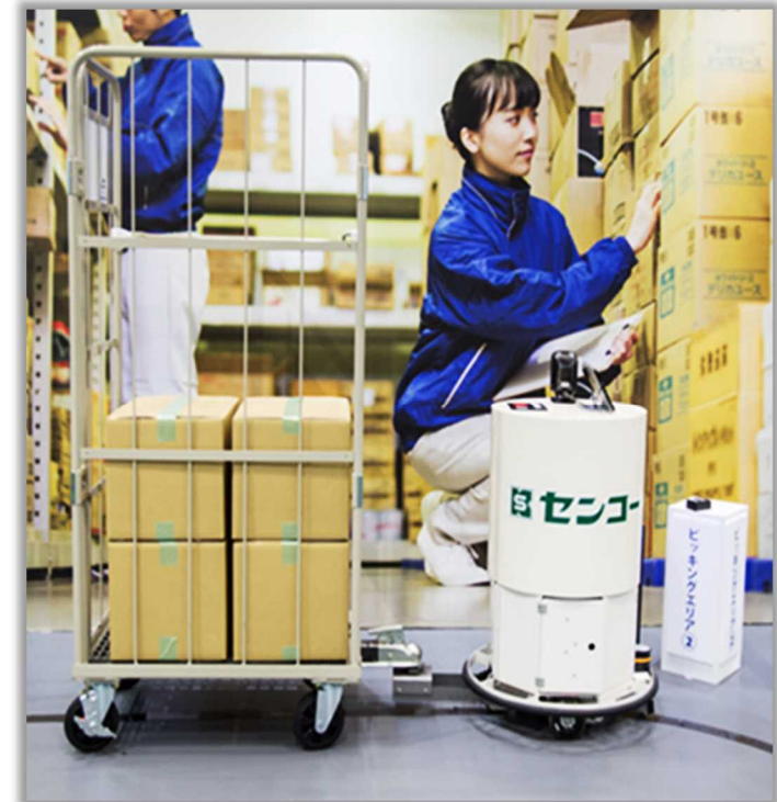
AGV capable of towing 500 kg
