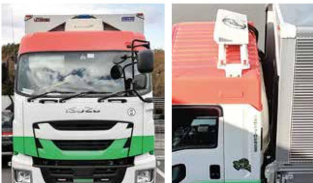
Truck equipped with "storage type cabin cooler" to support idling stop initiatives
