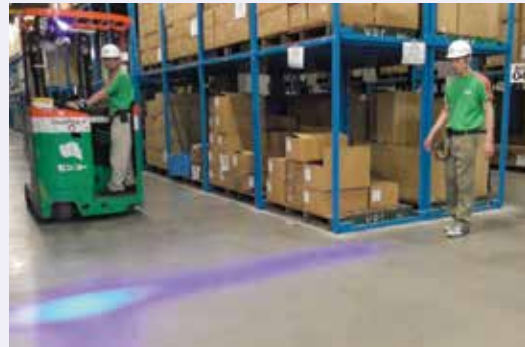
Avoids collisions between forklifts and walking workers
