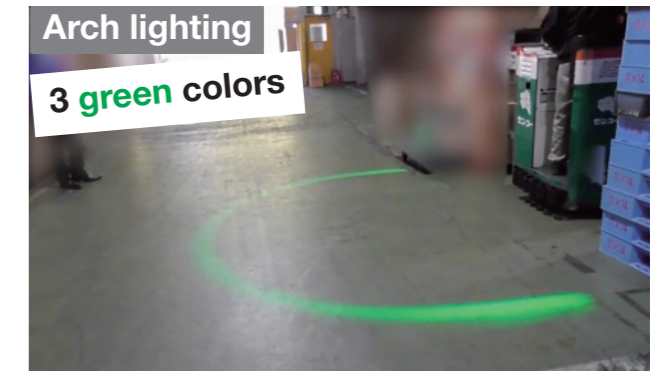
Avoids collisions between forklifts and walking workers
