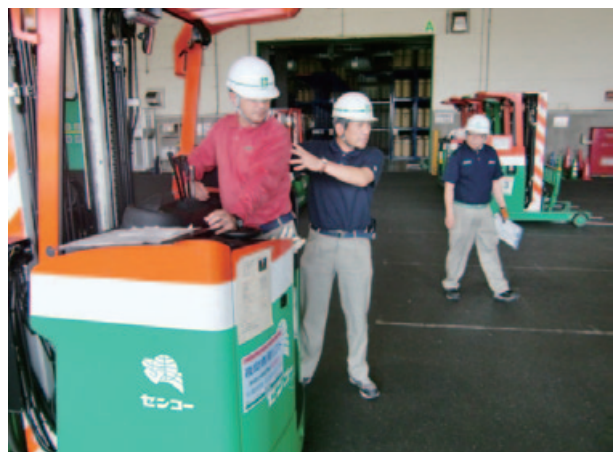
Instruction in points of caution when backing up a reach-type forklift truck
