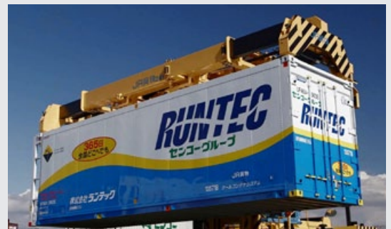
Original container with seismic isolation to prevent damage to delicate foods
