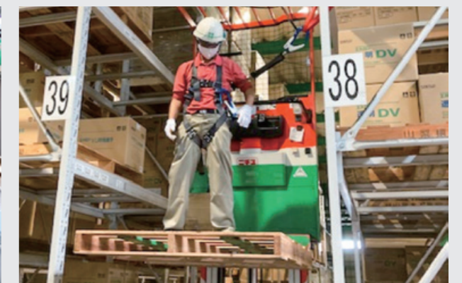
Practicing the correct way to fit devices to prevent from falling over
